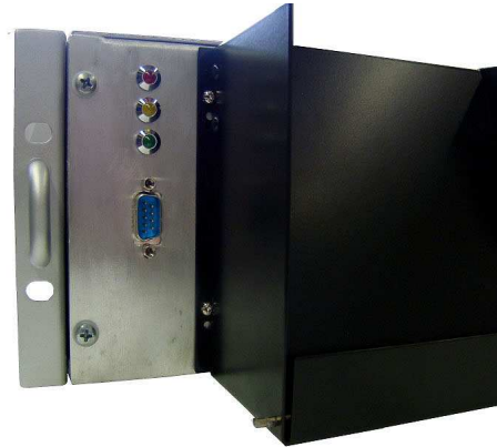
Front with status indicators and com-interface
